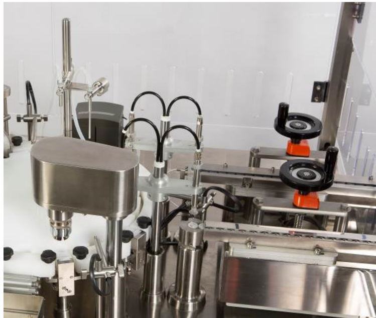
Pick and place capping unit with 180° movement at the end of a linear cap feeder
